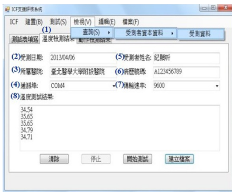
Figure 24 Query results of temperature detection. (Figure Translation: (1) 溫度檢測結果: The result of temperature detecting, (2) 受測日期: Date, (3) 所屬醫院: Name of Hospital, (4) 通訊埠Port, (5) 受測者姓名: Subject's Name, (6) 病歷號碼 Record ID, (7) 傳輸速率 Baud rate, (8) 溫度測試結果 The result of temperature detection).
