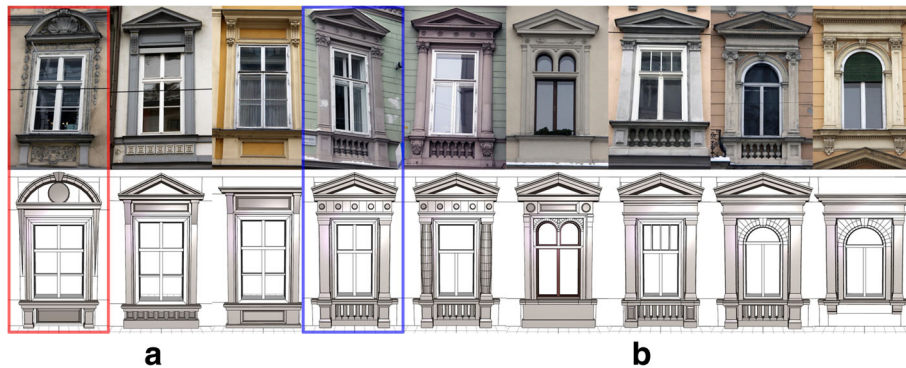
Fig. 3 Generative Building Blocks. Modeling of a family of similar structures can be facilitated using a generative approach, shown by this architectural example (Thaller et al. 2013): representative windows, respectively highlighted by a red and blue border, are modeled using a scripting language. Variations of these window types are generated by only replacing assets and adjusting proportions
