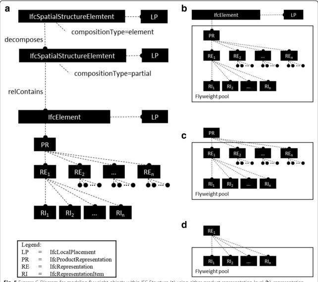
Fig. 5 Express-G Diagram for modeling flyweight objects within IFC Structure (a) using either product representation level (b), representation level (c) or representation item level (d)
