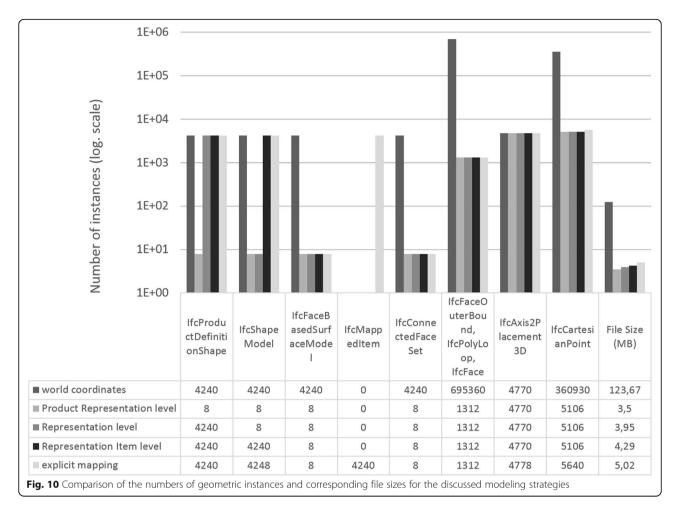
the eight segment types, which is why there exist eight additional instances of IfcShapeModel. Then it utilizes an IfcMappedItem for each segment, which for the whole tunnel results in 4240 occurrences. Furthermore, the number of placements and corresponding points increases, which is caused by the individual transformation of mapped items. Concluding the instance comparison, all numbers are reasonable with respect to the selected strategy.
